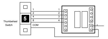
Note that Input #4 is the most significant bit and Input #1 the least significant bit. Next construct a ladder diagram using the [LDHex] function as follow:
