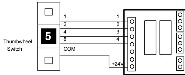
Note that Input #4 is the most significant bit and Input #1 the least significant bit. Next construct a ladder diagram using the [LDHex] function as follow:
