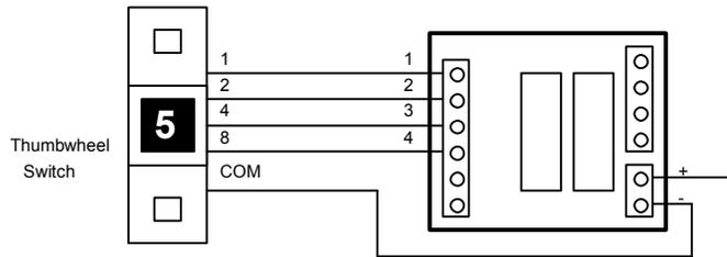
Note that Input #4 is the most significant bit and Input #1 the least significant bit. Next construct a ladder diagram using the [LDHex] function as follow:
