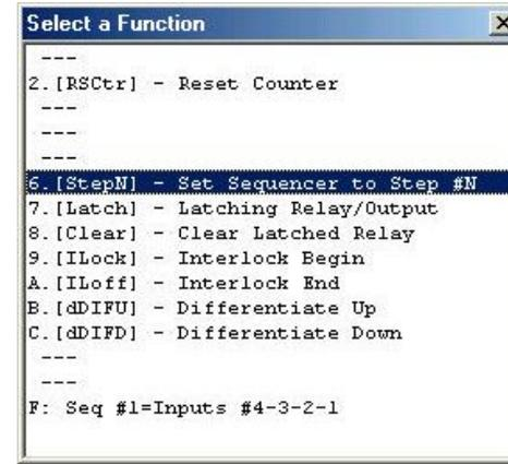
The Special Function menu will only show those special functions which are available to E10+ PLC. Those functions that are unavailable are replaced by the "--" symbol.
