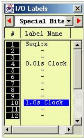
Unlike the H-series PLC which supports 8 sequencers, the E10+ PLC only supports 1 sequencer and two clock pulses.
